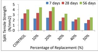
Fig. 3 Split tensile strength of concrete at various replacements at 7, 28 and 56 days
